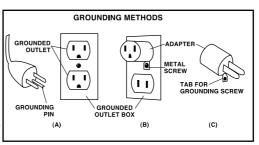
(sketch A) can be installed by a qualified electrician. The green colored rigid ear, lug or the like extending from the adapter must be connected to a permanent ground such as a properly grounded outlet box cover. Whenever the adapter is used, it must be held in place by a metal screw. Make sure that the appliance is connected to an outlet having the same configuration as the plug. No adapter should be used with this appliance.
